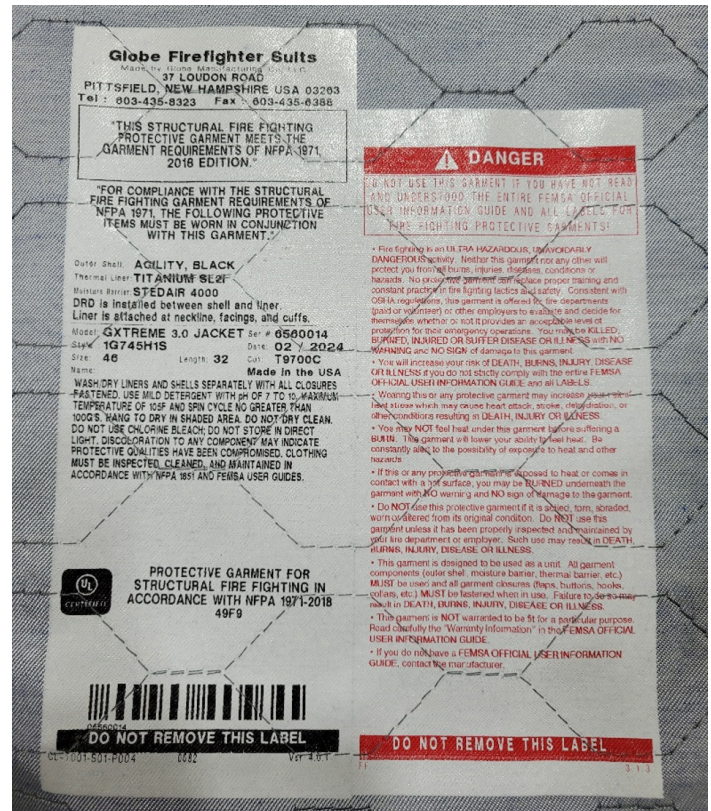
Current label on certified garment that is likely to change based on NFPA 1970 consolidation, but will still reference NFPA 1971.
